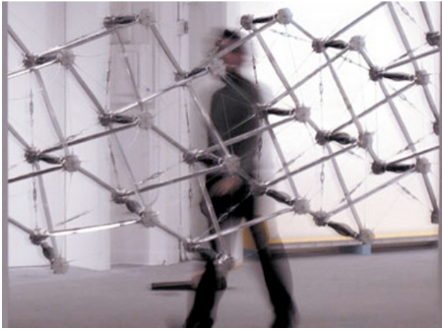
Figure 3. A prototype of an actuated tensegrity structure, courtesy of oframBFRA [4].
